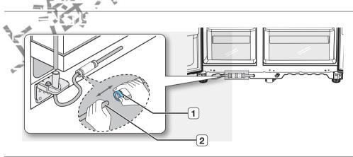
Do not cut the water line. Gently separate it from the coupler.
